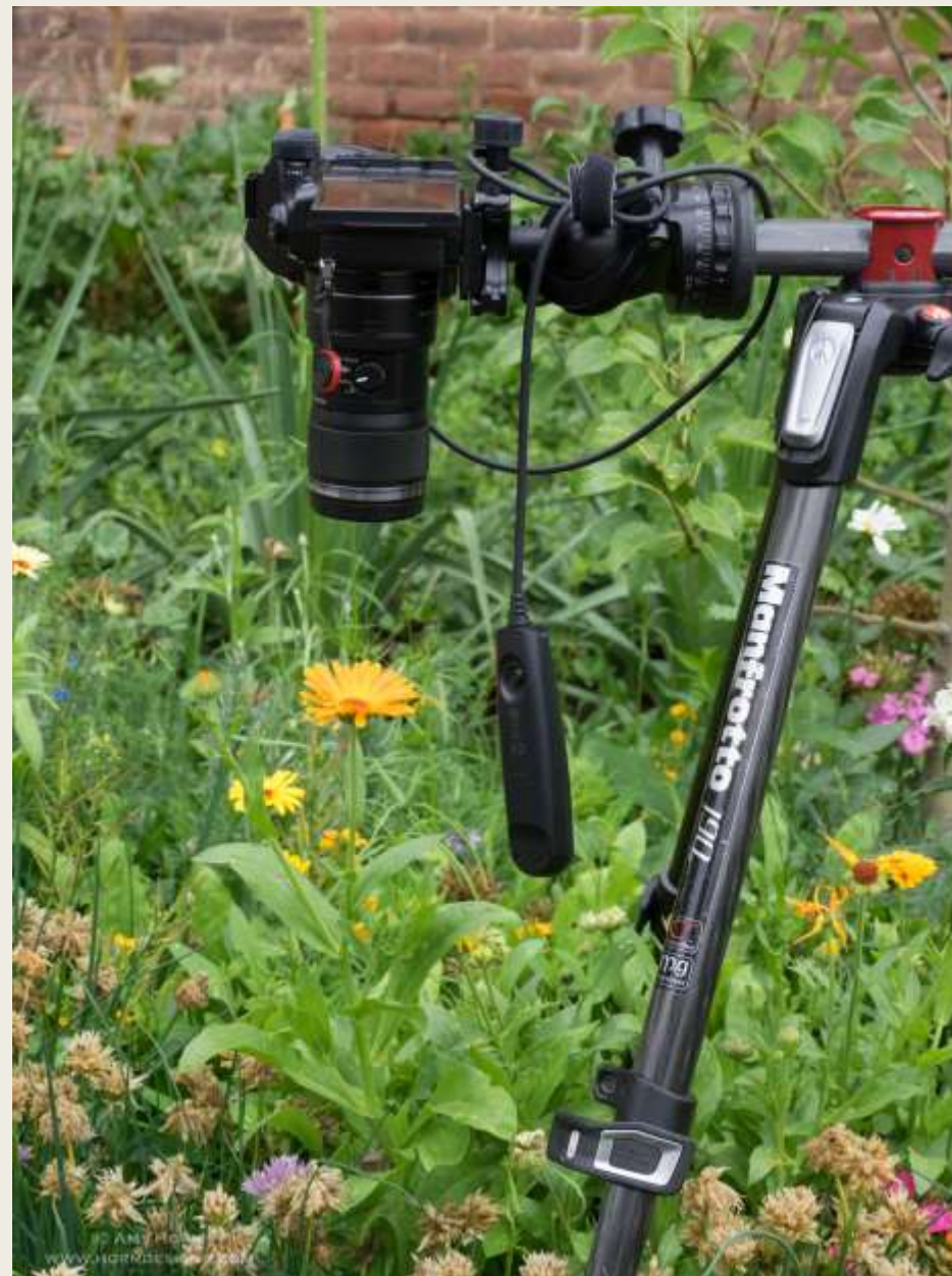
Macro lens with 26mm extension tubes
